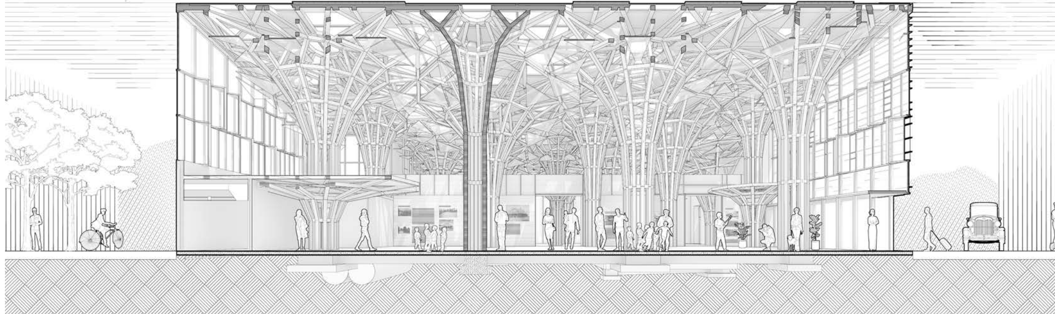
Top to bottom: In the Greenville: Rethinking Repair integrated studio, Huihui Dai, Yichen Wang, and Weisheng Zhong employed a dendriform structure to evoke the experience of walking in a forest in their design of a mixed-use building for a mountain community ravaged by wildfire. ☺ In their project "The Living Node" for the Component Assembly studio, Jiries Alali and Marian Roselem propose a flexible residential typology to densify the residential neighborhoods of Los Angeles.
